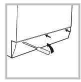
2. make sure the water level inside the machine is lower than the door opening; if it is not, remove excess water using the drain hose, collecting it in a bucket as indicated in the figure. 3. using a screwdriver, remove the cover panel on the lower front part of the washer-dryer (see figure).
