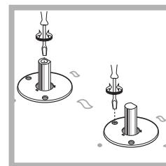
2. Remove the knob and adjust the adjustment screw, which is positioned in or next to the tap pin, until the flame is small but steady.
