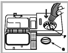
1. Open the dispenser by turning the lid (G) in an anticlockwise direction.
