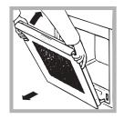
3. Grip the door on the two external sides and close it approximately half way. Pull the door towards you, lifting it out of its slot (*see diagram*).
