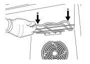
**2.** To return the heating element to its position, lift it up, pull it slightly towards you and make sure that the tab support is in its proper seating.
