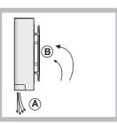
**AIR** maximises air circulation, improving the efficiency of the evaporator and helping to achieve the optimal temperature inside the refrigerator as quickly as possible each time it has been opened. The blown air (A) is cooled when it comes into contact with the cold wall, whereas the hotter air (B) is sucked up (see diagram).
