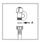
1. Insert seal A into the end of the inlet hose and screw the latter onto a cold water tap with a 3/4 gas threaded opening (see figure).
