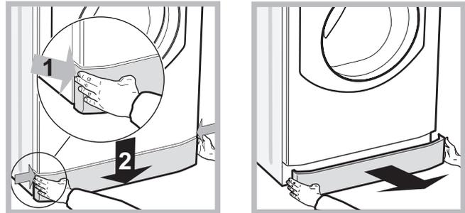
1. take off the cover panel on the front of the machine by first pressing it in the centre and then pushing downwards on both sides until you can remove it (see figures);
