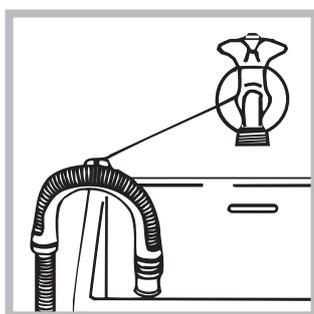
Alternatively, rest the drain hose on the side of a washbasin or bathtub, fastening the duct supplied to the tap (see figure). The free end of the hose should not be underwater.
