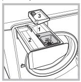
can be used with or without bleach. If you desire bleaching, insert the extra tray compartment (3) into compartment 1. When pouring in the bleach, be careful not to exceed the "max" level marked on the central pivot (see figure).
