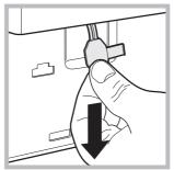
6. reposition the panel. making sure the hooks are securely in place before you push it onto the appliance.
