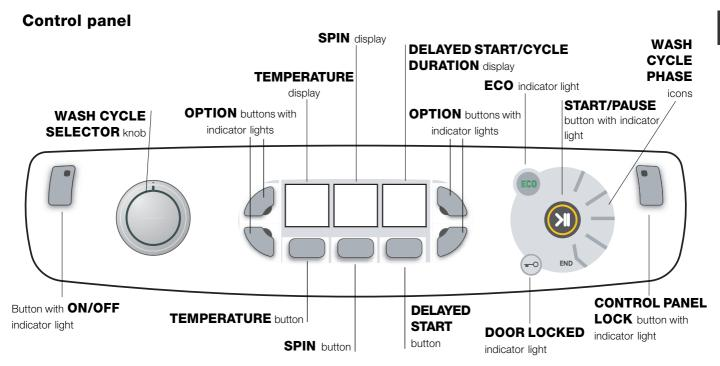
Button with () **ON/OFF** indicator light: press this briefly to switch the machine on or off. The green indicator light indicates that the machine is switched on. To switch off the washing machine during the wash cycle, press and hold the button for approximately 3 seconds; if the button is pressed briefly or accidentally the machine will not switch off. If the machine is switched off during a wash cycle, this wash cycle will be cancelled.
