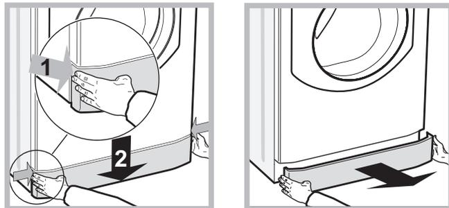
1. take off the cover panel on the front of the machine by first pressing it in the centre and then pushing downwards on both sides until you can remove it (see figures);
