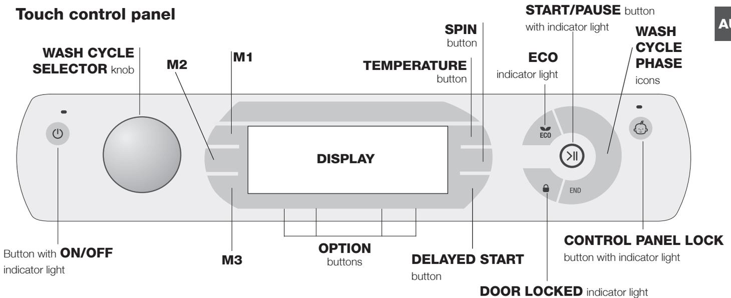
**Button with ON/OFF indicator light**: press this briefly to switch the machine on or off. The green indicator light indicates that the machine is switched on. To switch off the washing machine during the wash cycle, press and hold the button for approximately 3 seconds; if the button is pressed briefly or accidentally the machine will not switch off. If the machine is switched off during a wash cycle, this wash cycle will be cancelled.
