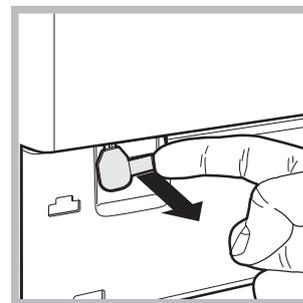
4. pull outwards using the tab as indicated in the figure, until the plastic tie-rod is freed from its stop position; pull downwards until you hear a “click”, which indicates that the door is now unlocked.
