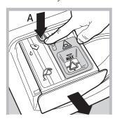
In order to fill the detergent and fabric softener tanks, the detergent dispenser drawer must be fully extracted: open the dispenser drawer up to the first stop point then press the lever (A) and open up to the second stop point, making sure that it is fully extracted. Avoid moving the dispenser drawer during
