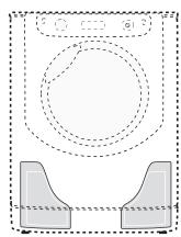
This washing machine is equipped with two tanks: one for liquid detergent (either concentrated or diluted) with a capacity of approx. 5.5 I and another for liquid fabric softener (either concentrated or diluted) with a capacity of approx. 3.5 I (see picture). I Check the detergent/fabric softener box to verify whether it is diluted or concentrated detergent. The automatic dosing system intakes the
