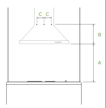
A **Minimum** height from the hob surface to the underside face of the rangehood **600mm** electric hob **650mm** gas hob – from top of trivot
