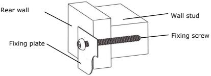
**1.** Pre drill pilot holes in the positions given (pg 4 - Installation position). Fix the fixing plate using the screws supplied or appropriate wall fixings, check with a spirit level to ensure bracket is level. Tighten screws.
