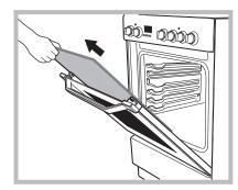
5.Remove the glass sheet and do the cleaning as indicated in chapter: "Care and maintenance".
